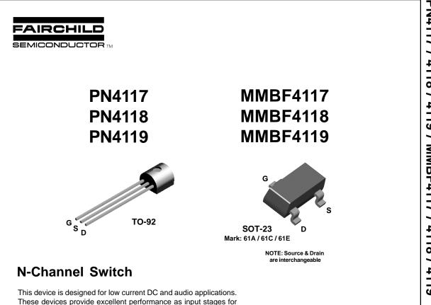
These devices provide excellent performance as input stages for sub-picoamp instrumentation or any high impedance signal sources. Sourced from Process 53.
